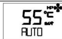
**Turning the appliance off:** simply press the ON/OFF button to turn the water heater off. The "SMILE LED" turns off, as does the DISPLAY light and other previously active signals; only "OFF" appears on the display. The protection against corrosion is still ensured, while the product will automatically ensure that the temperature of the water in the tank does not fall below 5 °C.
